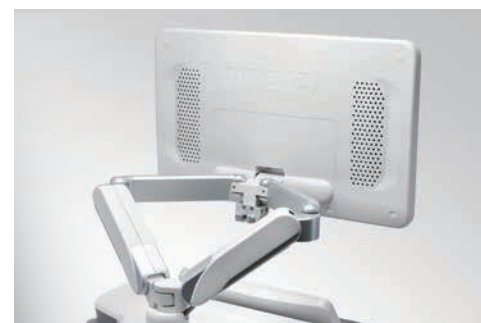
Unique dual-wing floating arm(optional)
