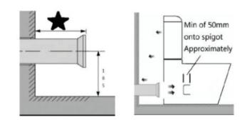
Step 2: Do the below installation for the cistern fixing.
