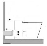
\*Align and push toilet pan back to the wall. Bucket flush and check for leaks.
