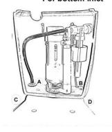
Remove cap from cistern plug A or B at base cistern. Connect flexible hose to cistern plug A or B depending on location of stop tap. Complete stop tap connection to underside of cistern plug A or B. Fill cistern and ensure correct water level. Note: Inlet valve can be adjusted if required.
