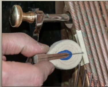
Action adjusted so #1 Hammer hits the strike point correctly
