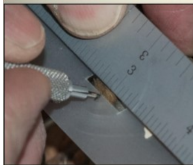
Notch Mylar strip to clear brackets
