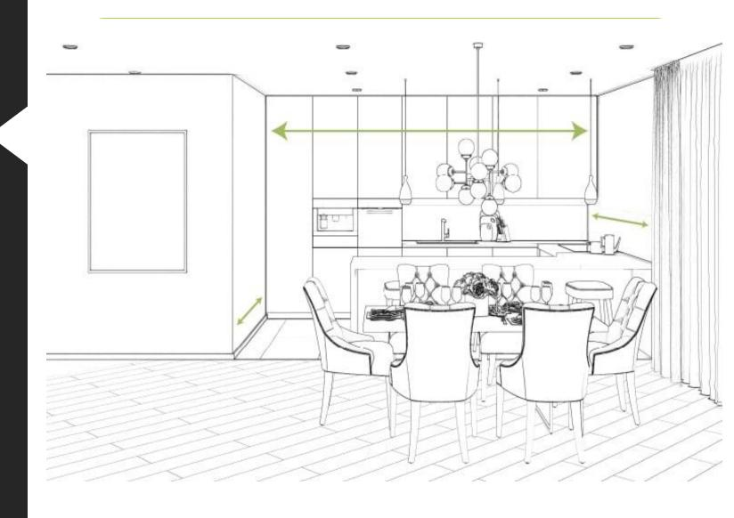
OMeasure the dimensions of fixtures, such as doors and windows, and how far they are from the walls, floor and ceiling (remember to include the frames in your measurements).
