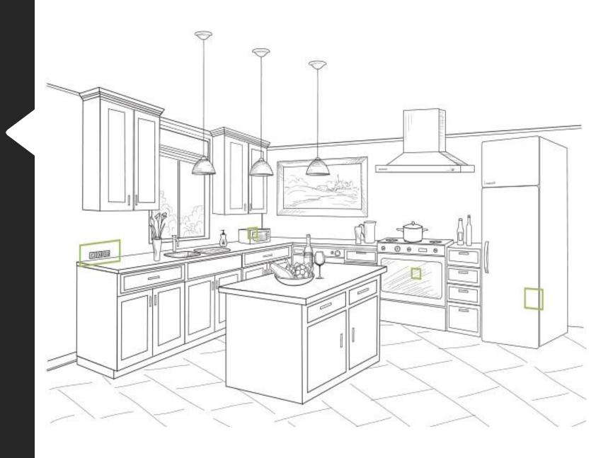
OJot down anything that sticks out into the room, such as ventilation shafts and pipes. Note the position of your drains, water supply and other plumbing points. If you are planning to relocate these, mark their new positions.
