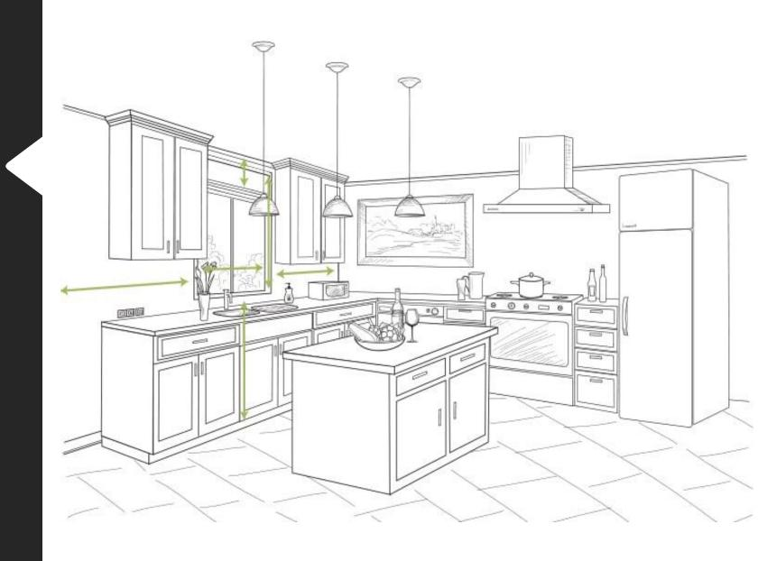
OSketch all plugs, light switches, light fixtures, stove and other electrical points that need to be marked (if you plan on relocating them make a note of the new positions on your diagram).
