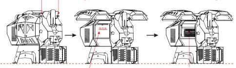
Remove the heat insulation plates on both sides
