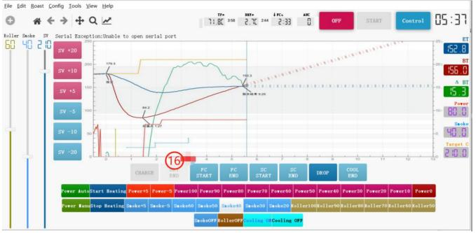
(1) adjust "Power", "Roller" and "Smoke"multiple times during the roasting process and click "DROP" at 10:36. The artisan system automatically turn on the cooling fan, then open the bean exit door
