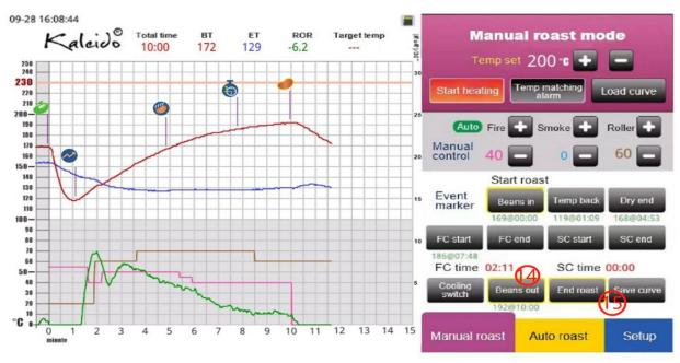
(15) Click indicate the end of cooling. Curves stop updating and you can continue to view the whole roasting date includes event node temperature @time. While Click save curve, you can save your roasting curve for future reference or use for automatic roasting.
