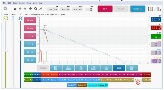
①Use the "Smoke" button to set the desired exhaust smoke speed The blue curve indicate the exhaust smoke speed change processes
