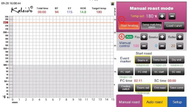
**5**The preheating curve is displayed at the far left of the curve pane. The preheating phase curve is not important, so we only have 30 second window so you can observe the temperature change situation within 30 second.
