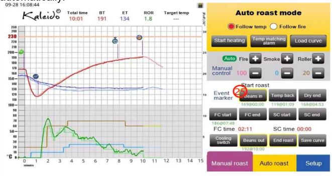
Next, using the same operation to mark events as manual roasting or not mark, including the "Beans out", "End roast" and "Save curve"
