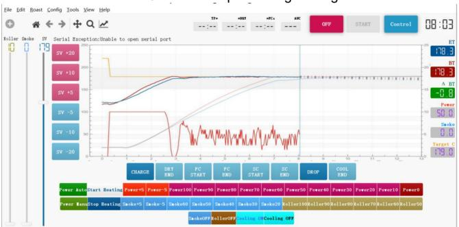
7When fully preheating, Click "CHARGE", then immediately open the bean entrance door and pour green beans into the drum, then close the door The system automatically adjusts the heating power to follow the curve according to the background curve bean temperature
