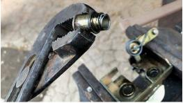
b. If you have difficulty prying out the old posts: drill out each latch post from the back side of the latch. Start with a 3/8" drill bit, and slowly enlarge the hole until the posts drop out, using 25/64" and 13/32" drill bits if needed.
