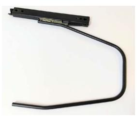
Once you have the sliders securely fastened to the seats you can secure them to the tracks in the vehicle. If your van is equipped with swivels you can bolt directly to the swivel tracks or remove the swivel and bolt to the tracks beneath it in order to reduce the seat height further.
