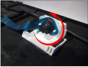
5. Installation of instrument cluster is reverse of removal. Test bulb operation before FULLY re-installing the instrument cluster (if a bulb does not function, twist it 180° to reverse polarity). If this does not work, check that the contacts on the new bulbs are protruding out far enough to make contact. If not, bend them out gently with a small screwdriver or pick so they make good contact with the foil.
