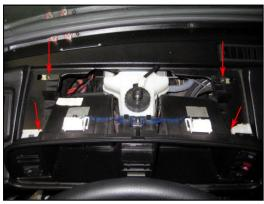
4. Place the instrument cluster face down on a table and carefully remove the 4 illumination bulbs. **Be** careful when removing these bulbs; the foil they contact can be very delicate. Gently untwist them from their sockets, and replace them with the new LED bulbs in the same manner.
