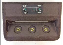
Note: It is extremely easy to break the console. It is recommended that you use a step drill bit to avoid fracturing the console.
