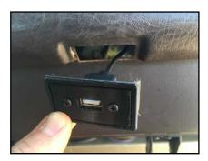
**7)** Insert one wing of the faceplate through the slot in the dashboard.
