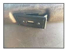
**8)** Bend the face plate to fit the wing on the opposite side into the slot. It may take some force!
