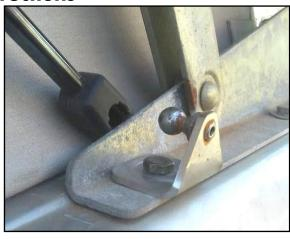
🖊 NOTE: It may be necessary to loosen all three bolts that hold the pop-top hinge to the body in order to get the bracket to fit. Mark the location of the hinge on the body in case the hinge moves—so you can put it back where it was. Masking tape works well for this.
