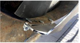
7) Torque down all bolts until the self-clinching stud heads are flush on the inside edge of the shroud opening.
