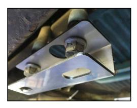
**4)** Place the M12x50mm bolts with washers in the bracket as shown in the diagram on the next page. Thread on the jam nuts. They do not need to be tight against the underside of the bracket. Thread a flange nut onto the right M12 bolt to the desired height, as shown.
