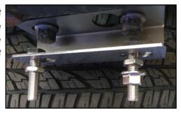
5) Test fit the spare tire by hooking the carriage over the flange nut. Lower the tire and adjust the jam nut and flange nut as necessary. When they have been adjusted so the tire is held snugly, tighten both flange nuts completely.
