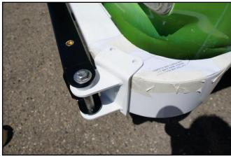
7) To mark the holes on the bottom of the bumper, with the M8 bolts tightened down on the top, open the arm and pull down to gain some leverage and make sure the bracket is snug up against the bumper. Mark the holes, remove the upper bolts, and complete assembly and drill out the holes. Reinstall the hinge and install the top and bottom M8 bolts.
