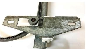
11. Use the window crank to drive the window mount plate fully on the window regulator guide rail. Ensure that the upper regulator guide is properly aligned on the guide rail.
