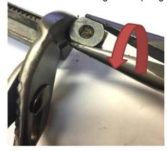
5. Hold the regulator spring firmly with a pair 6. Place the new pivot slider guide on the round pivot. Use two pairs of pliers to thread the round pivot point clockwise three turns back onto the regulator spring.
