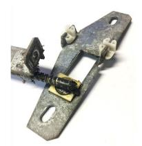
With the regulator spring free from the guide channel, thoroughly clean both the regulator spring and the guide channel to remove old grease and dirt. Lubricate these parts with high quality grease to ensure smooth operation of the window regulator.
