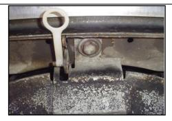
2) Next, remove the small retaining clips that hold the spare tire spring bars in place. Using a drift or drive pin punch, tap the ends of the spring bars out of the tire carrier, and remove the spare tire carrier from the vehicle. Rotate each of the retaining springs so that the front bent ends can be removed from the vehicle.
