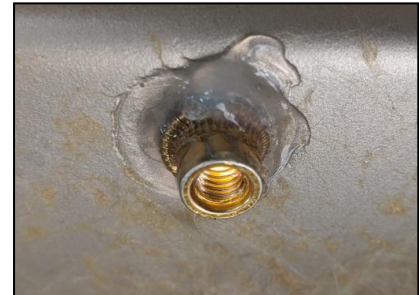
Installed Rivnut as viewed from inside the van
