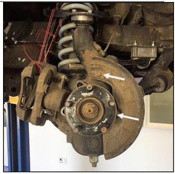
**5)** Slide the flap onto the steering knuckle and secure the dust shield with the provided 18mm long 6mm bolts with washers. The bracket will line up with the dust shield mounting holes. If your dust shield is missing or worn out, be sure to check out GoWesty's new dust shields online.
