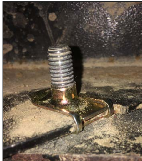
View of clip nut from inside the bumper
