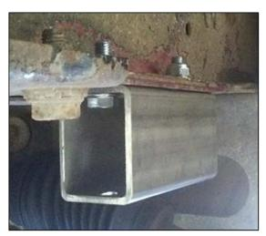
2) Install the sway bar with the rubber bushing and strap. Send the 8mm bolts through the strap, making sure to include the thick washers. Repeat for the other side.
