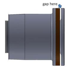
Figure 2: 2WD arms that are too narrow will exhibit a gap between the inner sleeve and bushing when installed.
