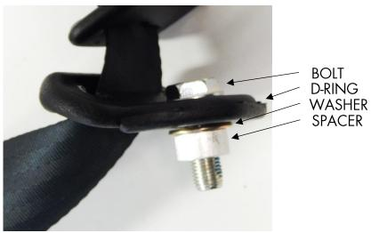
4. Install receiver, using the bolt, washer, and spacer provided, in the factory-threaded hole on inboard side of the seat pedestal where the original receiver was mounted. The washer is placed between the bolt and the receiver, as shown below. Torque bolt to 45-55 ft-lbs.
