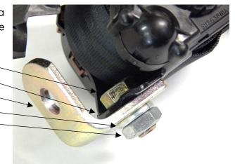
2. Install the inertia reel and the belt end next to the seat, utilizing the existing threaded hole and original hardware. Torque bolt to 45-55 ft-lbs. (In passenger buses, with the heating duct in the door, the reel must be oriented with the bulge facing outboard.)
