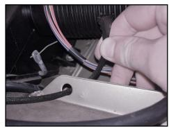
2) Insert the ball end of the other strap firmly into the slot on the right side.
