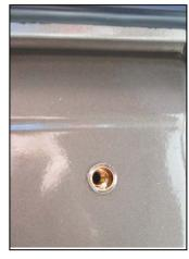
With the rivnut in place, reattach the awning and brackets to the gutter. Bolt down the bottom bracket with the M6x20mm screw, using the included rubber washer to protect the van's paint. Tighten the 5/16" nut to secure the bracket around the gutter. While tightening the bracket, try to keep the inner bracket over the thicker portion of the pinch weld inside the gutter.
