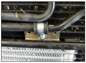
The long hose runs between the cooler and the thermostat. Cut a small section of the shroud between the radiator and the body of the vehicle to pass the hose through. You can add some large rubber hose or other material around the hoses here to protect against abrasion if necessary. Be sure to leave enough length in the hose to allow the cooler to be tilted forward, along with the whole radiator assembly, when it is tilted out during service appointments.
