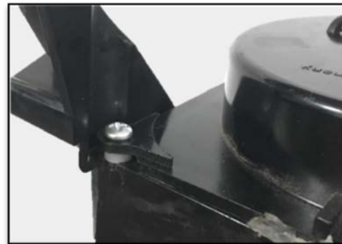
Gauge Corner Repair
