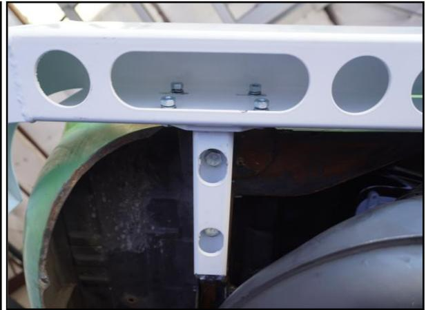
**⚠** NOTE: Volkswagen specified a tongue weight of 100 lbs for their original trailer hitches. While our bumper is Class III in strength, we rate it to Class I (100lb tongue weight/1000lb tow rate) as we feel it is unsafe to tow anything over 1000lbs with a stock bus. We do not recommend doing so or you will risk damaging your frame rails.
