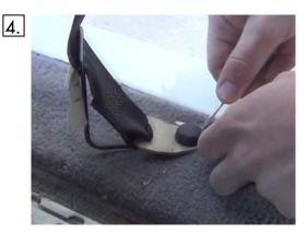
Remove the bolt cap, and bolt to remove the belt end from the seat pedestal
