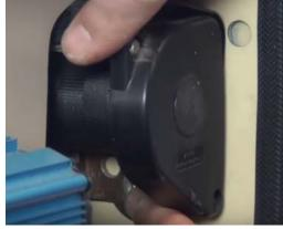
Pull the webbing out of the reel to easily access the bolt. Remove the bolt, and unsnap the cover to provide enough room to wiggle the reel out.
