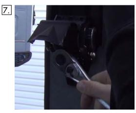
Bolt the new reel in, taking care to ensure it is vertically straight. Torque the reel bolt to 35 lb-ft
