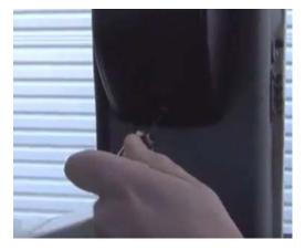
Begin by removing the phillips head screw to release and remove the plastic shroud over the reel. Your van may not have this cover. 2.
