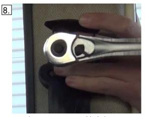
Unsnap the D-Ring cover and bolt the D-Ring in place. Be sure the mounting hole is squared on the shoulder of the bolt, so it pivots freely. Torque to 35 lb-ft
