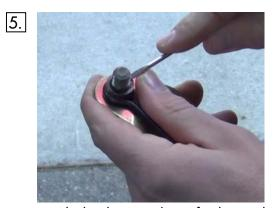
Remove the hardware and save for the new belt. The plastic ring may need to be cut or pried off to remove the hardware.
