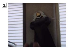
Remove the D-Ring. You will need to remove the cover to access the bolt.
