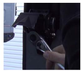
Unsnap the reel cover, and remove the 17mm bolt holding the reel. You may need to unreel the webbing to fit a wrench or socket in place
