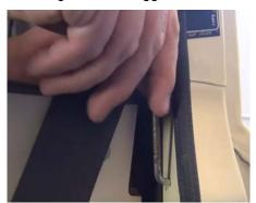
Rotate the guide bar up and pull it out.
