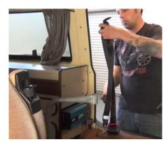
Install your new belt in reverse of removal. Torque all bolts to 35 lb-ft.
