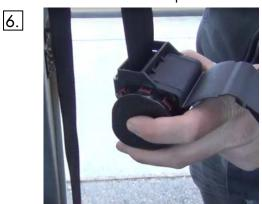
Remove some slack from the new reel. It will not unravel unless it is in an upright, vertical position.
