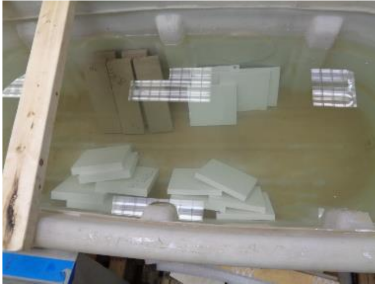
Photo No. 3 ASTM C97 Absorption Testing
