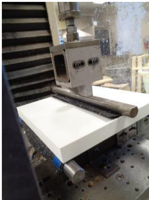
Photo No. 4 ASTM C1505 - Breaking Strength (3-point load) - Test Setup
