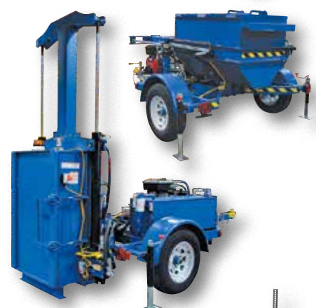
Crushes 55 gallon steel drums to only 6" high.
