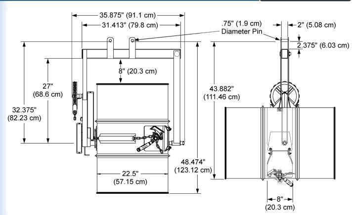
NOTE: Standard loop of pull chain extends approximately six feet below the chain wheel
