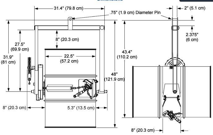
NOTE: Standard loop of pull chain extends approximately six feet below the chain wheel. Custom lengths are available.
