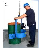
Secure drum holder to your drum between drum ribs... no tools are needed. To secure drum, drape the cinch chain with flexible chain cover across the front of the drum, insert one link into the slot on the ratchet handle, and turn the ratchet handle clockwise to tighten the cinch chain around the drum.
