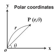
**Example**> Determine the polar coordinates  $(r, \theta)$  when the rectangular coordinates of Point P are (x = 7, y = 3).
