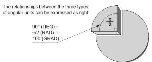
Angular values are converted from DEG to RAD to GRAD with each push of the key (2nd function of ). This function is used when doing calculations related to trigonometric functions or coordinate geometry conversions.
