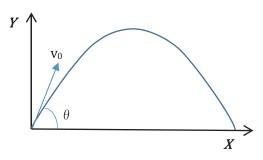
(1) Assuming an initial velocity of 20 m / s and an angle of 40 °, check the transition of height and distance after x seconds. (g=9.8)
