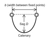
When a = 0.846 and b = 2, find the rope sag D and the rope length L.
