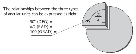
**Example>** Check to confirm 90 degrees equaling  $\pi/2$  radians equaling 100 grads. ( $\pi$ =3.14159...)
