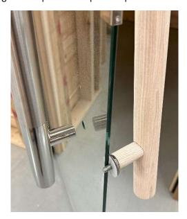
Push screw through bottom hole in the glass, and swing the metal handle out to apply both spacers. Partially tighten bottom screw; make sure handle is straight from top to bottom and finish tightening screws to complete installation.
