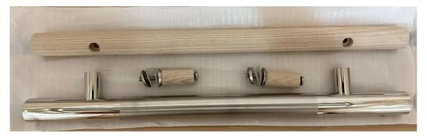
Install both wood spacers into wooden handle. Insert screw into wooden handle through the spacer and place metal spacer and plastic spacer over screw. Insert screw through the top hole in the glass from the inside, so the wooden handle is inside the unit.
