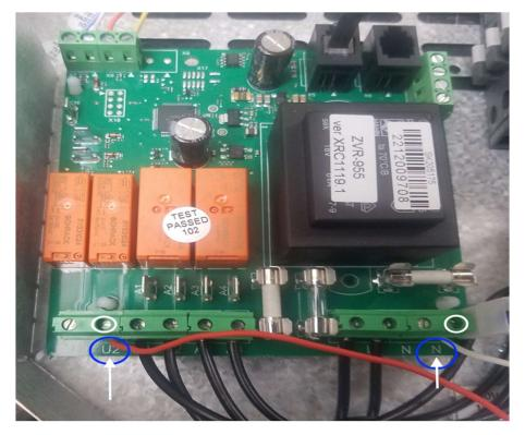
Output wires from U2 and N will run to a dedicated 120V outlet to operate the sauna lighting. Wiring diagrams can be found in the Xenio CX manual and under the top cover of the power box, but here is one for reference.
