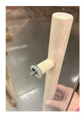
Now place the plastic spacer and metal spacer over the screw. Mate the metal handle to the screw on the outside of the unit, and partially tighten screw. Swing handle to the side to access screw. Repeat process from above by applying metal spacer and plastic spacer over screw.
