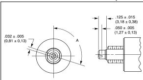
Series 56 rotary switches are available with a screwdriver slotted shaft with dimensions as shown. Available in the styles, angles of throw and pole/positions combinations shown in the choice and limitations chart.
