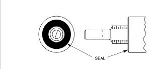
Panel is sealed by a flat rubber seal washer at the base of bushing. Shaft is sealed by an Oring inside the bushing. After the switch is mounted, seals do not alter the dimensions of the unsealed style.
