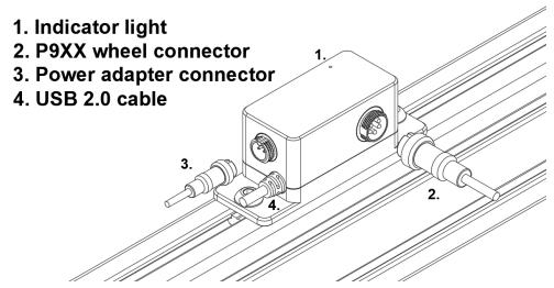
Indicator light out: No USB connection Indicator light blue: USB connection
