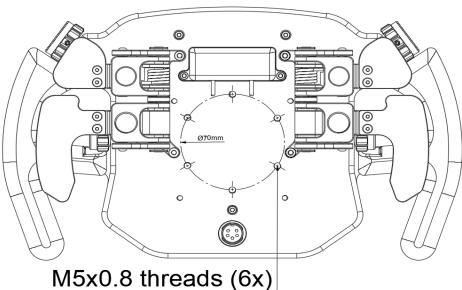
WARNING: When mounting a third party wheel hub, the bolts connecting the hub to the P9XX Sim Racing Wheel, cannot exceed a length of 12mm + wheel hub flange thickness. Example: The wheel hub flange has a thickness of 4mm, the total length of the M5 threads bolt cannot exceed 16mm. Using longer bolts can damage the screen.
