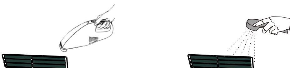
If the filter screen is not too dirty, just use the vacuum cleaner to absorb the dust.
