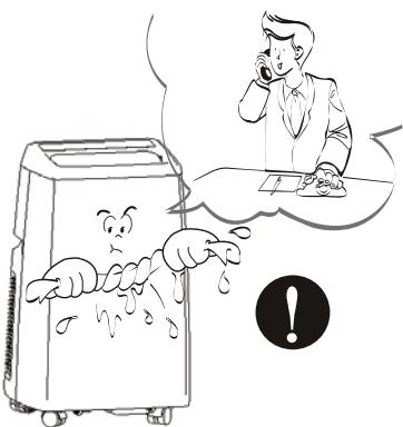
If you need to wipe, clean, move the machine or replace the machine parts, please turn off the machine and unplug the power plug first.
