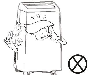
If water enters the machine, shut it down immediately and pull out the plug, then contact the professional maintenance personnel for repair.
