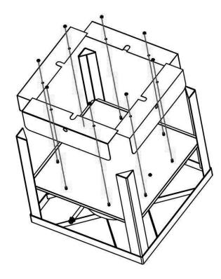
3. Assemble the (4) small heat plates to the large heat plate with bots/nuts.
