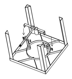
1. Assemble the jet burner to the base with bolts/nuts.
