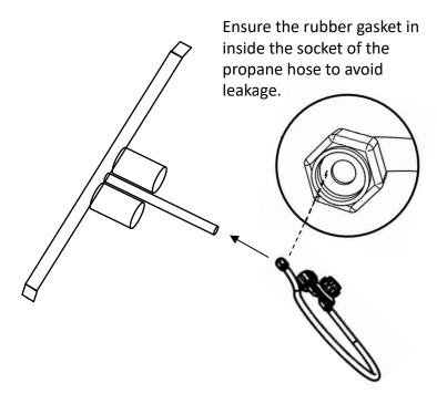
4. Connect the propane hose to the Jet burner as shown.
