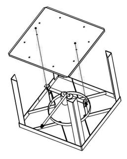
2. Assemble the large heat plate to the jet burner with bolt/nuts.
