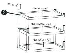
Step 3, Repeat steps 1 to complete the installation of the top shelf.
