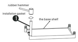
Step 1, Locate the base shelf, use rubber hammer and installation gasket to knock the aluminum tube into the slot of the four corners of the shelf, as shown in the figure 1, until the pipe calibration line is level with the slot plane.
