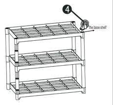
Step 4, Put the cart upside down,Insert the casters into the holes as shown in the figure 4.
