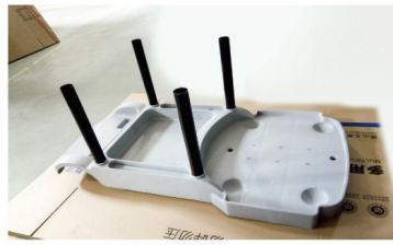
Put Pillar in the hole
