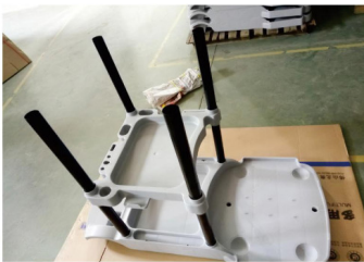
Put Pillar in the hole
