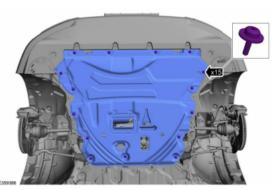
4. Remove the engine splash shield. This requires a T30 Torx bit. There are 15 screws in total. FX4 models need not remove entire skid plate, only remove those screws required to remove the bumper cover.
