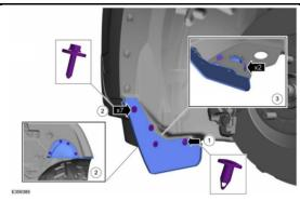
1. Remove the plastic air deflectors. This requires a 7mm socket for the screws and a small pry tool for the clips. To remove the clips, you must first raise the inner pin. With
