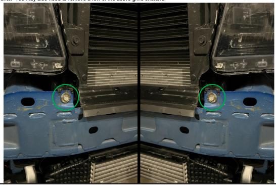
11. Using the supplied hardware, loosely assemble the light mount and attach it to the chassis as shown below, remember to reuse the two bolts previously removed. With the brackets mounted securely, you can now install your lights. Please note that space is tight where the lights will mount, so you may need to remove and reinstall the light bar to properly mount and aim your lights.
