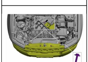
7. Remove the four screws that secure the upper grille as identified below.
