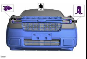
8. Release the clips that are behind the grille. These clips are built into the headlights, so be very carefully as not to damage the headlights.
