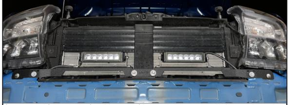
Once you are satisfied with the aim of your lights, you can fully tighten the light mount assembly. Make sure that your lights and all mounting points are secure. To reinstall the front bumper & grille, simply follow the removal steps in reverse.
