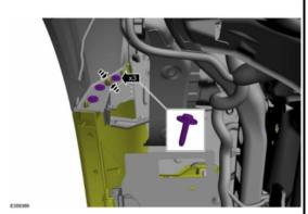
6. On both sides, remove the three bolts that secure the bumper cover to the fender. The bolts are 10mm. There is also a clip on each side that must be released as shown below.
