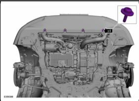
5. Remove the four screws securing the lower bumper valance. Also a T30 Torx.
