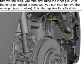
3. Disconnect the front bumper wiring harness. This is located on the passenger side and can be accessed from behind the fender liner
