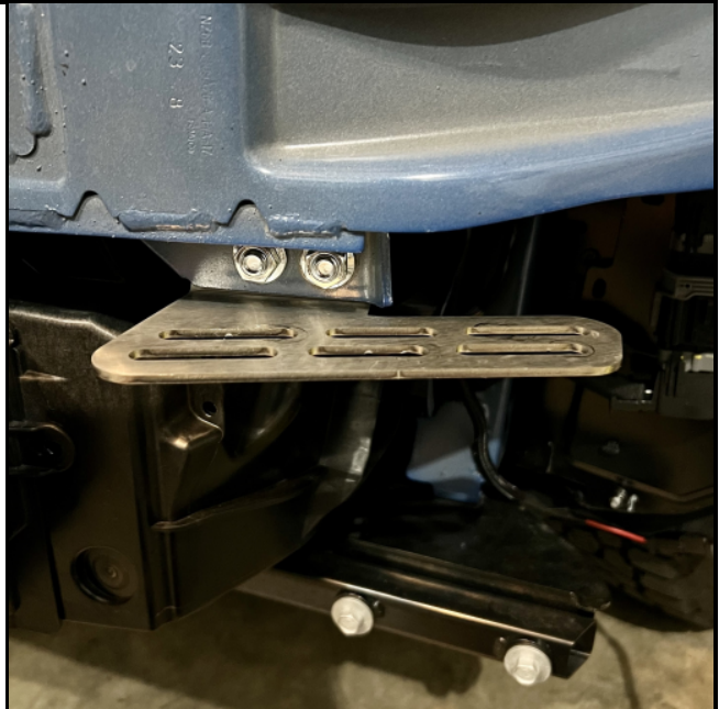
Driver Side Bracket Installed
