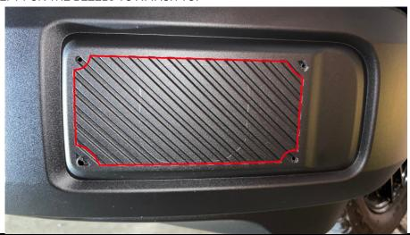
Once you have the openings cut, you can install the bezels with the included hardware. The bezels only need to be snug, do not overtighten the bezels.
