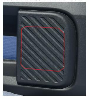
A hole template is also provided to help mark the outer corners that need to be drilled in order to install the bezels. For these holes,  $\emptyset 3/16$ " is all that is needed but  $\emptyset 1/4$ " drill bit will also work. Do not exceed  $\emptyset 1/4$ " holes.
