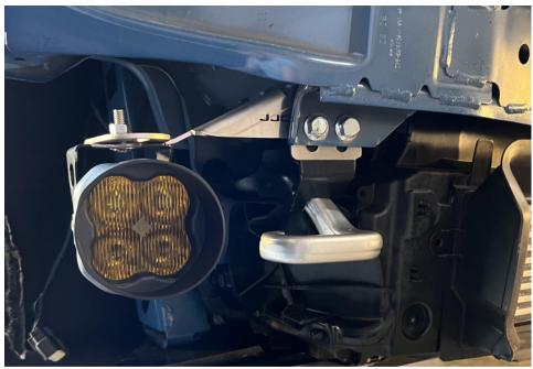
To install the brackets, remove the front tow hook bolts (12mm), insert the bracket and reattach the tow hook as shown. With the brackets mounted securely, you can now install your lights. (Passenger side shown above for reference)
