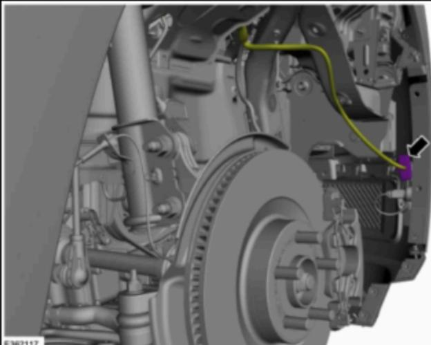
3. Disconnect the front bumper wiring harness. This is located on the passenger side and can be accessed from behind the fender liner
