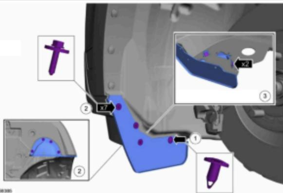
1. Remove the plastic air deflectors. This requires a 7mm socket for the screws and a small pry tool for the clips. To remove the clips, you must first raise the inner pin. With the inner pin raised or removed, you can then remove the outer pin (see 1 below). This step applies to both sides.
