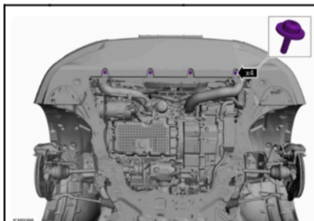
5. Remove the four screws securing the lower bumper valance. Also a T30 Torx.
