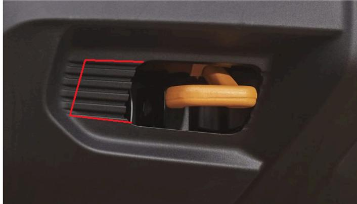
Completed installation of passenger side bezel shown below.
