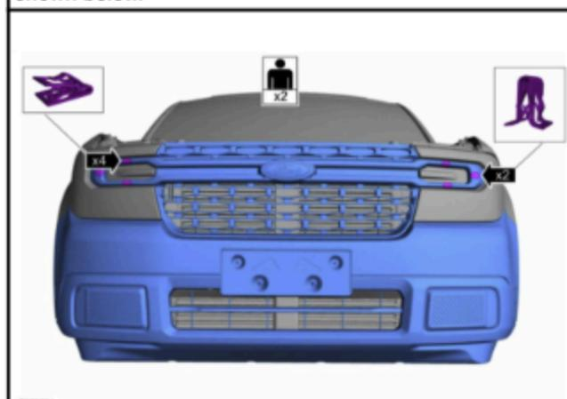
8. Release the clips that are behind the grille. These clips are built into the headlights, so be very carefully as not to damage the headlights.
