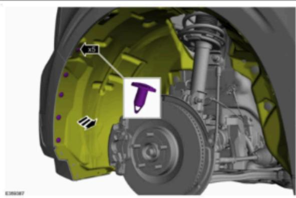
2. Remove the 5 push pins that secure the fender liner to the bumper cover and fender. Applies to both sides.
