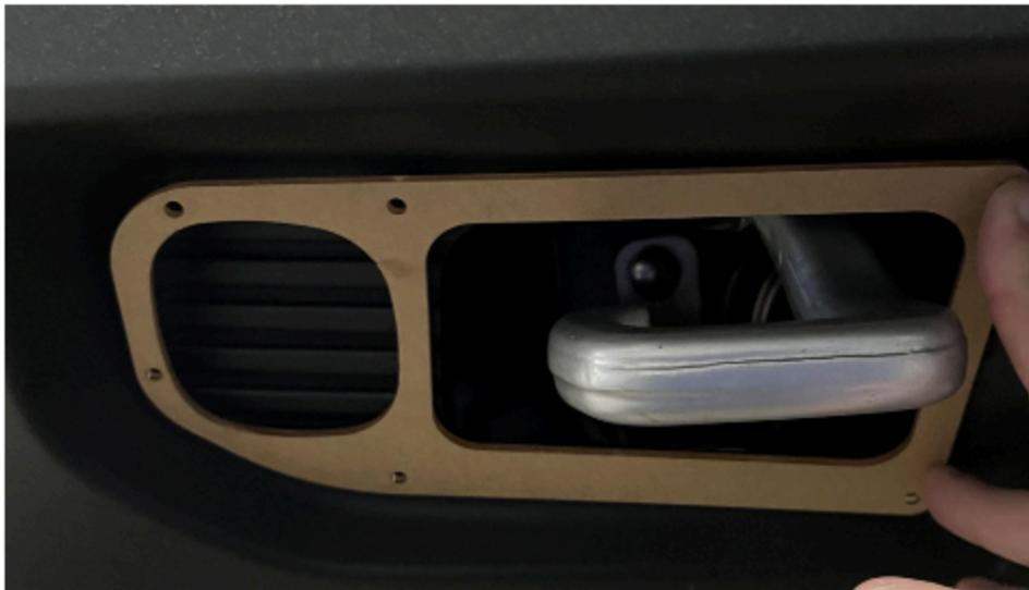
Using the included template, mark the fog light openings that need to be cut. Once marked, you can carefully cut the openings. Remember, it is easy to remove more material as necessary but it is rather impossible to add material back if you cut too far; so start small with your cutting and increase your opening size only as needed. The entire opening does not need to be cut, only cut what is necessary for your particular installation.
