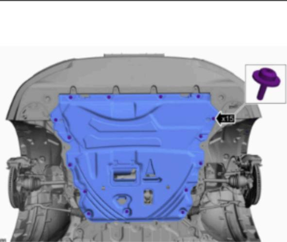
4. Remove the engine splash shield. This requires a T30 Torx bit. There are 15 screws in total. **Tremor models need not remove entire skid plate, only remove those screws required to remove the plastic bumper cover.**
