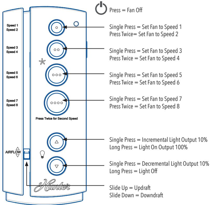
**NOTICE** Toggle dimming mode by holding OFF (⏻) and quickly press Light Down (▽) two times
