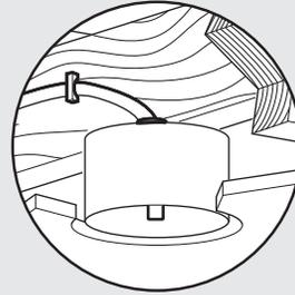
You must be able to secure the fan to building structure or fan-rated outlet box and clearly marked acceptable for fan support of 70 lbs (31.8 kg) or less.
