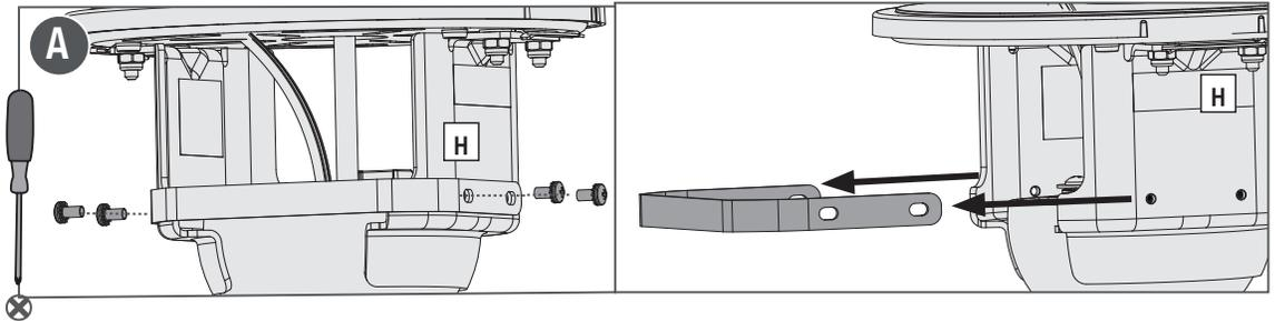
Remove any existing bracket prior to installation. Only use the provided Hunter ceiling bracket that came in your fan's box.
