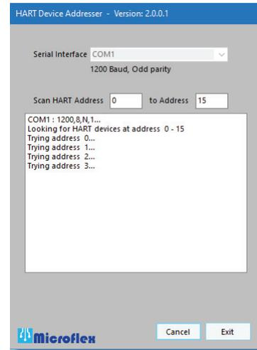
Figure 8. Scanning for a field device.
