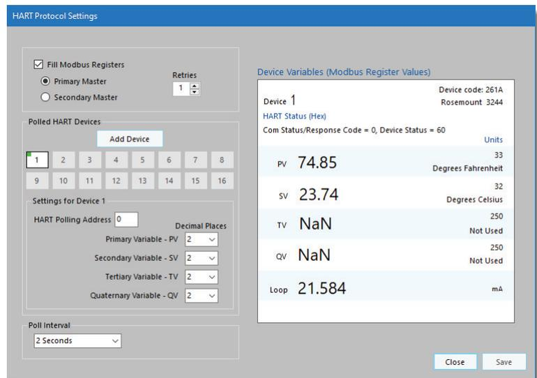
Figure 5. HART Protocol Settings (Fill Modbus Registers checked). Poll one HART field device, polling address 0, every 2 seconds.
