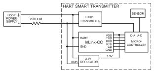
Figure 2. Typical Application, HART smart transmitter
