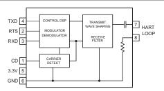
Figure 1. InLink Block Diagram
