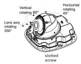
Step 7 (Arrange the cable of camera to over-line buckle, if the type of camera is inner-line), then assemble the dome cover with hex wrench, as shown in figure 3-4.
